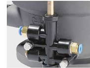
The position to install interlock valve
