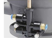
The position to install interlock valve
