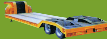
Semi Trailer Low Bed, Singapore YTE75 Suspension and 9500 Series Axle
