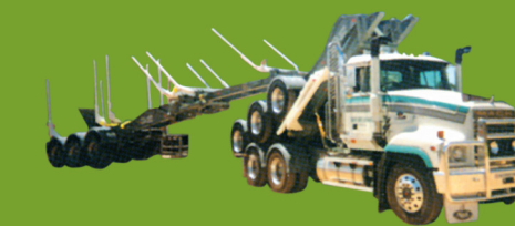
Port Semi Trailer, Singapore YTE75 HD Suspension, 2000 Series Axle and Self Steer Axle
