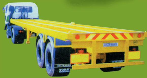
Semi Container Trailer, Bangladesh YTE75 Suspension and 2000 Series Axle
