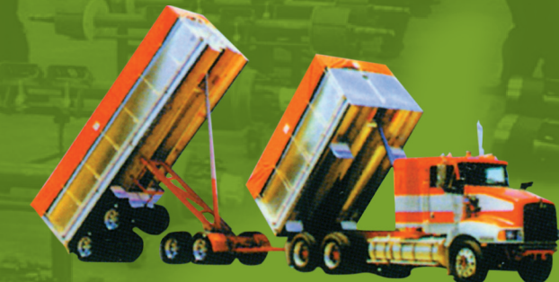
Dump Draw-Bar Trailer, Middle East YTE75 Suspension and 6000 Series Axle
