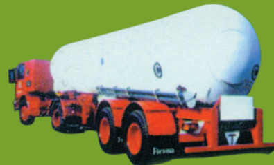
Semi Trailer Petrol Tank, Malaysia YTE75 Suspension and 2000 Series Axle
