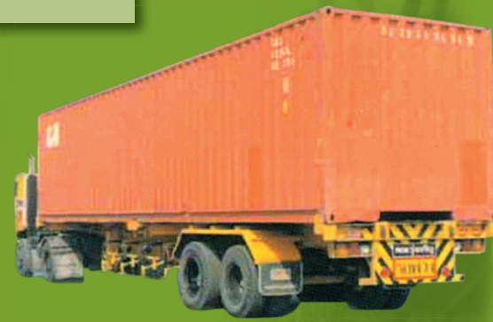
Semi Container Trailer, Thailand YTE75 Suspension and 2000 Series Axle
