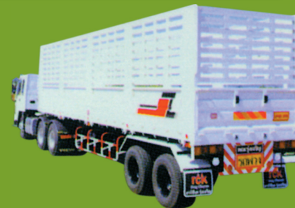
Semi Cargo Trailer, Thailand YTE75 Suspension and 2000 Series Axle
