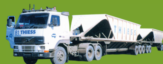
120 Tonnes Mining Trailer Train, Indonesia YTE90 Suspension and 8000 Series Axle
