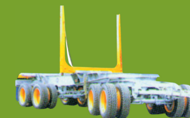
Port Semi Trailer, Indonesia YTE75/90 Suspension and 8000 Series Axle
