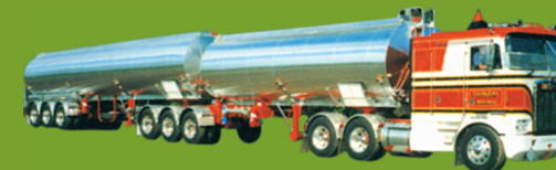
Petrol Tank B Double Trailer, South Africa Tecair I Suspension and TN Bearing Series Axle
